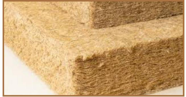
Thermal and acoustic wa floor & ceiling insulation in hemp fiber batt.
