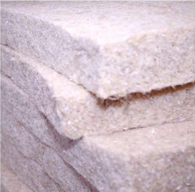
Thermal and acoustic wa floor & ceiling insulation in hemp fiber batt.
